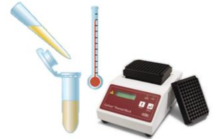
3 LYSE Add sample to BAX ® Lysis Reagent and heat to rupture cell wall and release DNA into solution.
