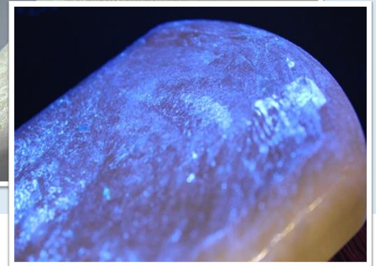
UV gel 'contamination' trapped in surface defects after cleaning
