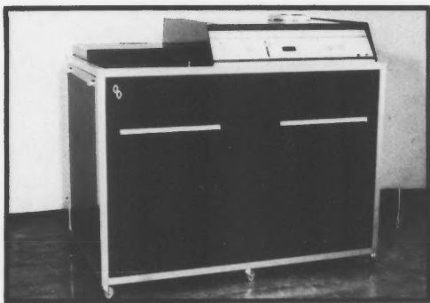
"The KJEL Foss Automatic is AOAC approved for the determination of crude protein."
