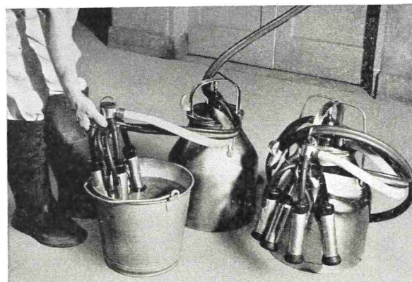
USE OF TRITON-HYAMINE IN PRE-RINSE solution is an effective way to obtain maximum sanitation of milking machine parts.
