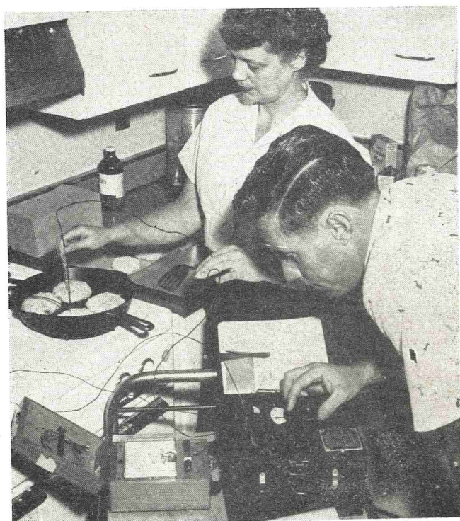
Figure 1. Copper-constantin (24-gauge) thermocouple wires inserted into crab cakes. The terminal ends are connected to a Brown Portable Potentiometer (Model 126 W3).
