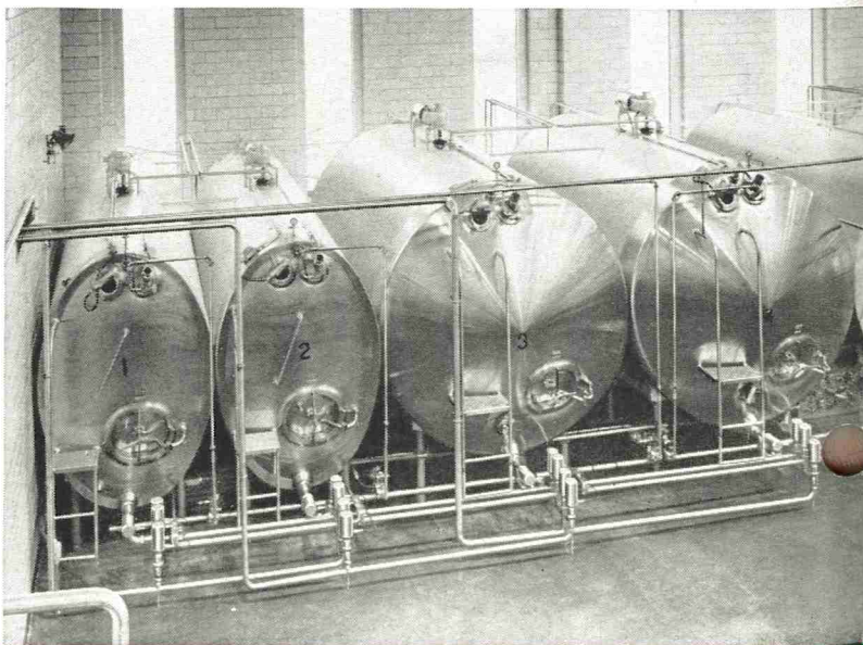
Tri-Clamp and Tri-Weld fittings couple Fesco valve manifolds and provide unrestricted flow and positive flow controls.
