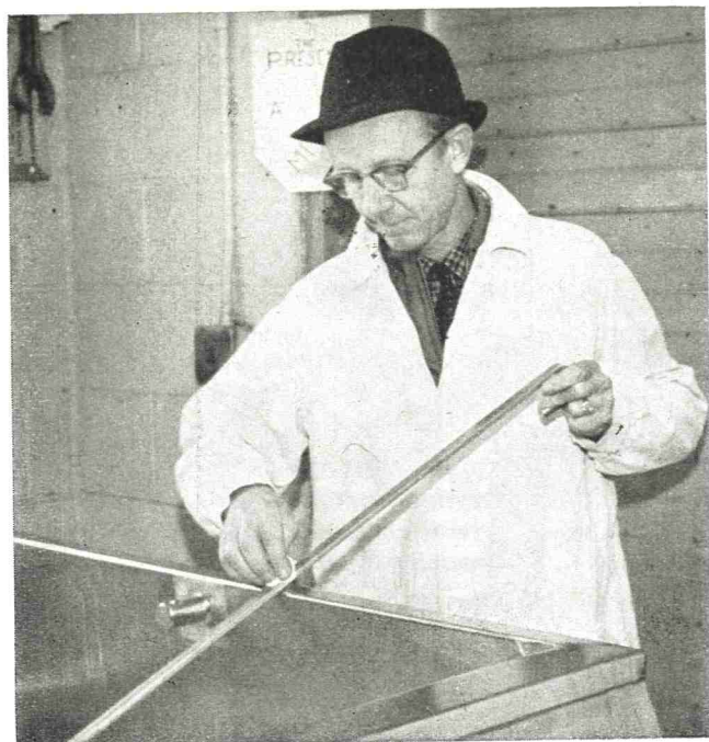
Figure 3. Demonstration of technique commonly used by milk collectors: remove rod from cold milk, wipe with tissue, reinsert, remove, read.
