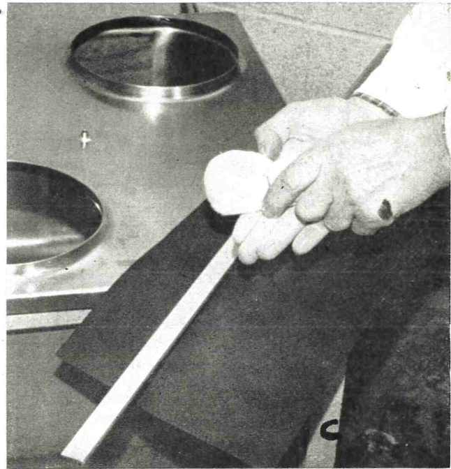
Figure 2. (A) Preparing gauge rod for calibration; (B) scrubbing rod preparatory to rinsing and drying; (C) "powdering" the rod just before calibration.
