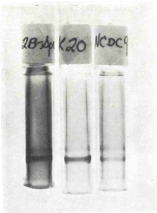
Figure 7. Typical esterase patterns for three strains of Vibrio parahaemolyticus . From left to right: Chesapeake Bay isolate, Zen-Yoji strain, and a strain of V. parahaemolyticus isolated from a U.S. tourist returning to the United States from a tour of the Far East (culture provided by the Center for Disease Control, Atlanta, Georgia). Details of procedures have been published (31).
