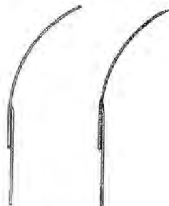
FIGURE 3 Early welded seam
