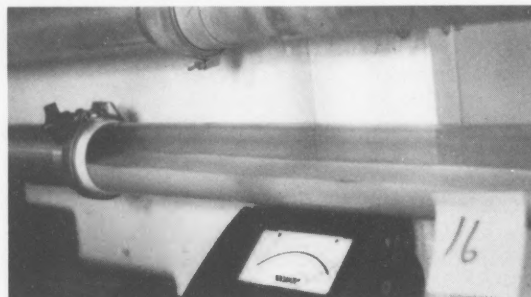
Figure 2. Transparent pipe installed in milk pipe prior to receiver entry with 16 units at maximum milk flow. Mark on pipe above meter is at 50% fill depth.
