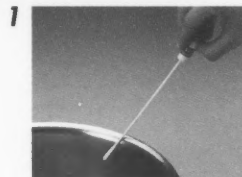
1 Wet the swab with Biotrace's unique swab moistening fluid and swab the surface in the normal way
