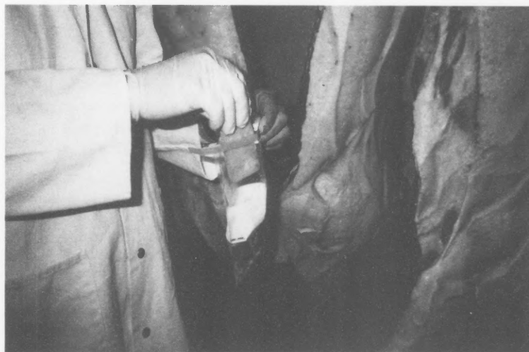
Figure 2-B. The sponge is transferred to the WhirlPak™ bag and transported to the laboratory.
