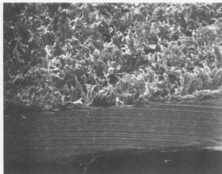
Figure 6. Sample F. Scanning electron microscopy of a HDPE link extracted from a conveyor system in a poultry processing facility where frozen nuggets had drapped onto the belt.
