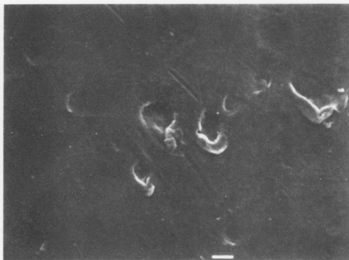
Figure 1. Sample A. Scanning electron microscopy of a new, unused HDPE conveyor link.
