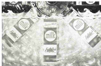
Cartons are immersed in pure, hot paraffin just seconds before being filled with milk... an exclusive Pure-Pak sterilizing feature!
