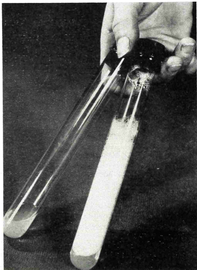
FIGURE 2. A minute amount of silicone preparation effectively eliminates foam in a soap solution.
