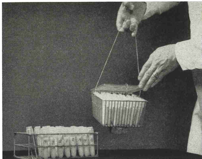
Figure 2.—Apparatus used in making laboratory pasteurization tests showing raw milk samples in plastic tubes and weighted covered wire basket.
