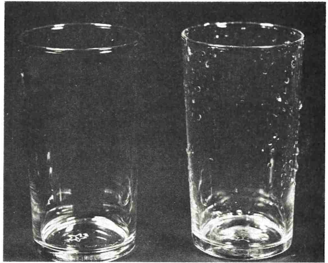
Figure 3. Comparison of two glasses with and without the use of rinse additive. On left, rinsed with 100 ppm additive to water; on right, rinsed without the use of rinse additive.
