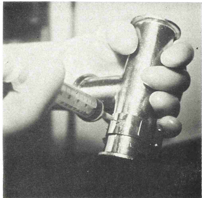
Figure 1. New sampler consisting of a 3/8-inch drilled hole with a soft rubber insert secured into place with stainless steel clamp. Sample taken with syringe.
