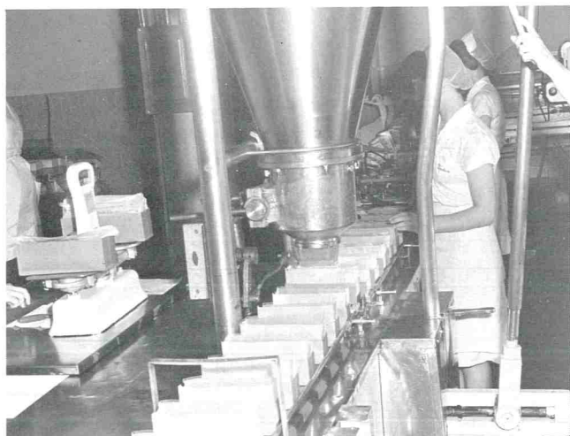
Figure 7. Filling 2-lb. paper boxes lined with semi-transparent, wax-coated Cellophane, circa 1940. (Courtesy of Borden Foods, Cheese Division, The Borden Co.).
