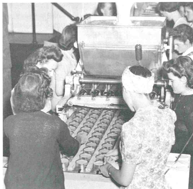
Figure 8. Filling 4-oz. tin cans with process cheese for the Armed Forces during World War II. (Courtesy of Borden Foods, Cheese Division, The Borden Co.).
