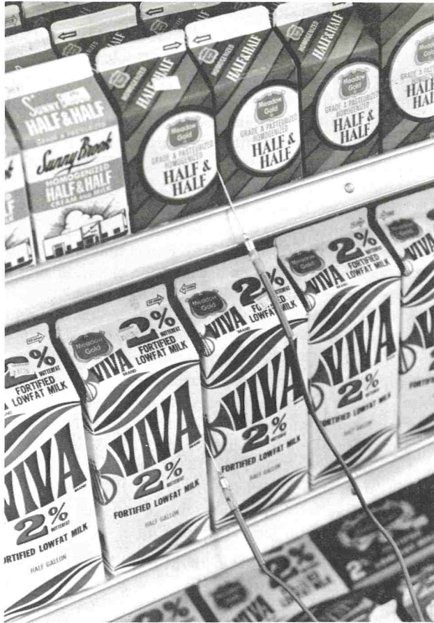
Figure 2. Placement of surface probes directly between the exterior surfaces of adjacent containers of product.
