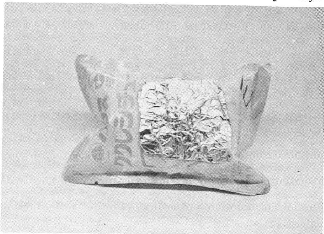
Figure 4. Clostridium sporogenes 7955 (P.A. 3679) inoculated retortable pouch containing vegetable soup after 4 days of incubation at 35 C.
