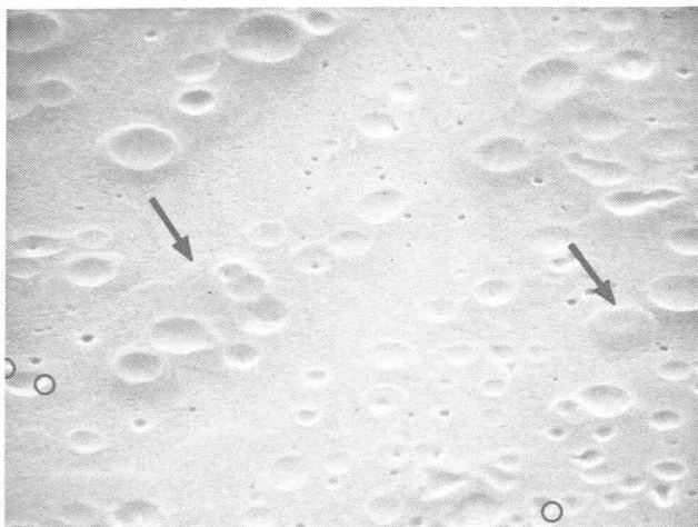
Figure 5. Scanning electron photomicrograph (1000X) of exposed and unrinsed whole milk film on stainless steel plates. Arrows indicate edges of layers formed from ruptured fat globules. Objects in circles are probably lactose granules.
