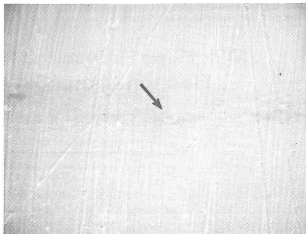
Figure 1. Scanning electron photomicrograph (1000X) of unexposed, rinsed plate surface. Arrow shows depth to which plate was immersed in whole milk.
