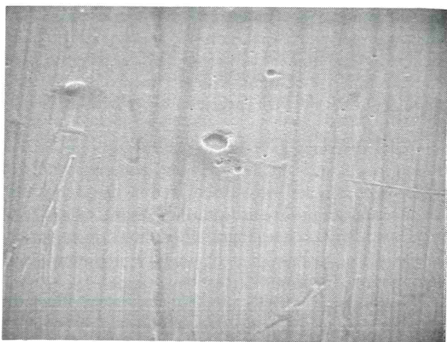
Figure 3. Scanning electron photomicrograph (1000X) of exposed and unrinsed skim milk film on stainless steel plate.
