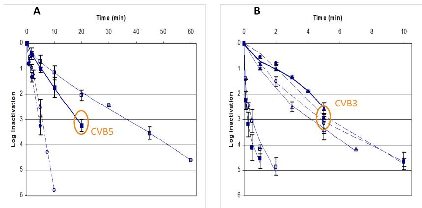
A: Free chlorine inactivation of coxsackievirus B5 (squares) and echovirus 1 (circles) B: Free chlorine inactivation of adenovirus 2 (squares), coxsackievirus B3 (circles), and echovirus 11 (triangles); closed shape = pH 7, open shape = pH 8
