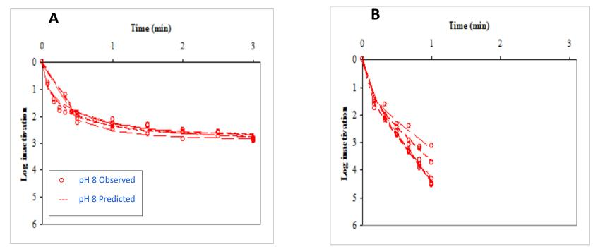
Inactivation curves for aggregated (A) and monodispersed (B) adenovirus type 2 in surface water with 0.2 mg/L free chlorine at 5 °C
