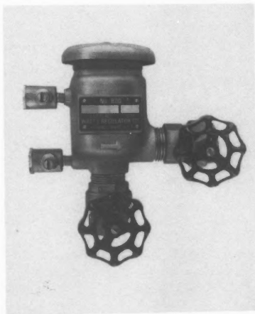
Figure 2. Pressure Vacuum Breaker. May be placed under continuous line pressure. Not suitable where backpressure may occur. Requires annual testing.
