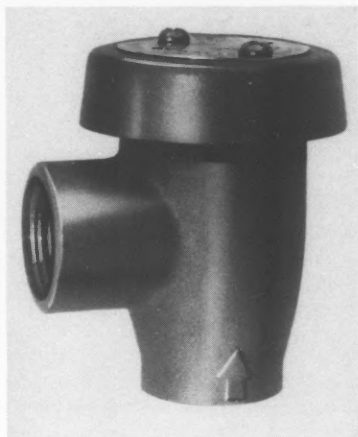
Figure 1. Atmospheric Vacuum Breaker. Cannot be placed under continuous line pressure. Not suitable where backpressure may occur.
