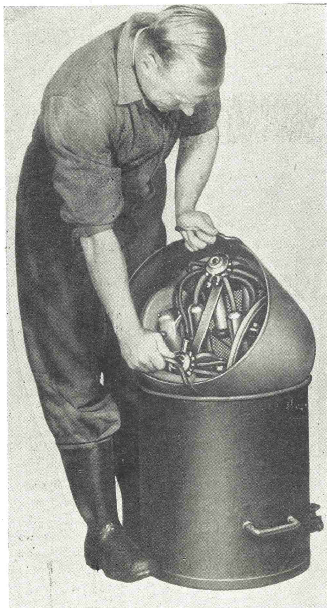
Figure 3. Apparatus used in the immersion cleaning method for direct-to-can milking machine equipment.
