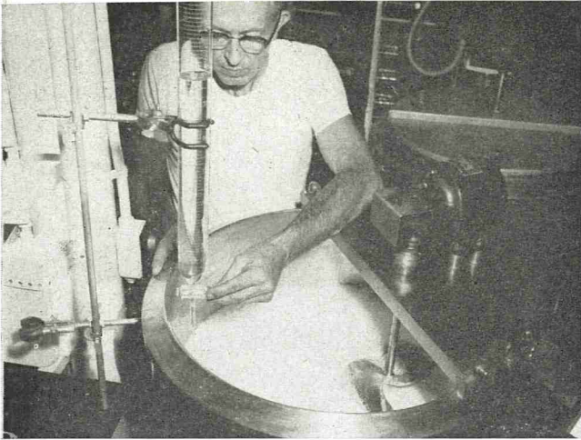
Figure 3. Scientists found that for efficient radiostrontium removal, they had to increase the acidity of the milk. Here USDA dairy technologist, Homer E. Walter adds dilute citric acid to the milk preparatory to passing it through the "fixed-bed" ion-exchange resin column. By thus lowering the milk's pH from its normal 6.6 to 5.4, the percentage of radiostrontium removed by the process is raised from 60 to 98.
