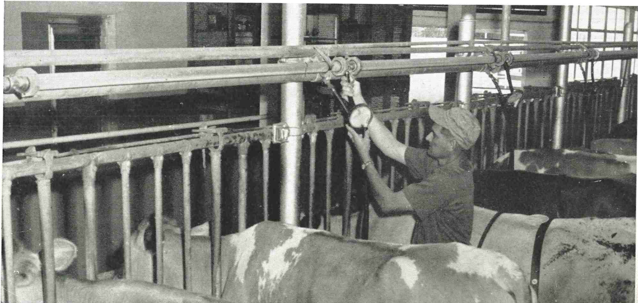
Cow-To-Can Operators —Milker tube attaches to inlet nozzle; outlet tube goes directly to can.
