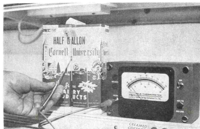
Figure 1. "Tele-Thermometer" equipped with surface probe accurately indicates internal product temperature from the outside without disturbing product.
