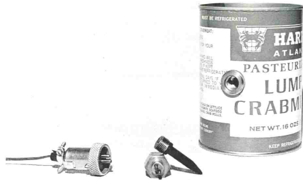
Figure 1. Instrumented can of crab meat showing thermocouple, packing gland, and connector.
