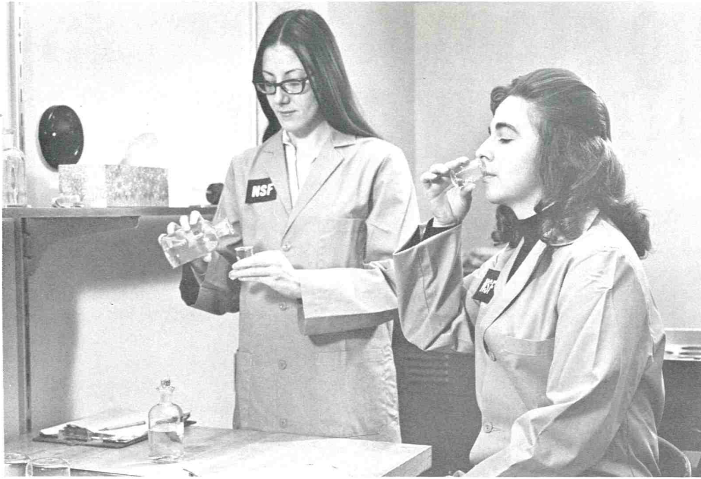
DRINKING ON THE JOB! Taste and odor testing of water—which has stood for test periods in plastic pipe samples—is required by NSF standards.
