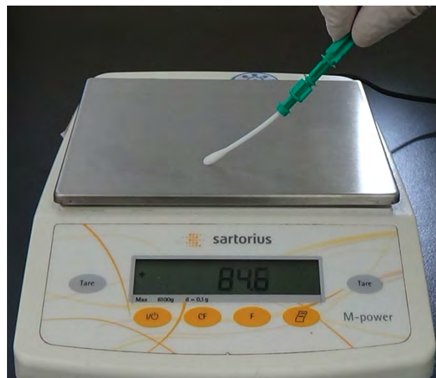
FIGURE 1. The measurement of swabbing pressure on the scale pan of the analytical balance using the A3 test swab. When the swab shaft slightly bent, the balance showed approximately 70–100 g.
