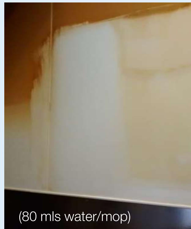
Microfibre mop used to clean greasy walls in a snacks production site
