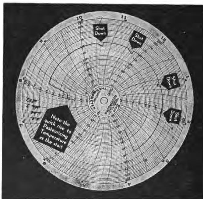
The thermal recorder chart shown above is a typical record taken from a CHERRY-BURRELL Isotherm Heater now in daily operation in a recent large installation. Note the quick, positive rise to pasteurizing temperature at the start, and the evenness of the line showing how this temperature was maintained—within tenths of a degree. Also note the *immediate* return to pasteurizing temperature when the milk flow was resumed after a shutdown while awaiting milk from storage.
