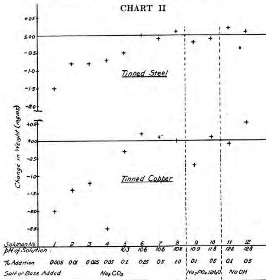
*Changes in Weight of Tinned Metal Strips Half Immersed in Hypochlorite Solutions (100 ppm Available Chlorine) for 48 Hours at 50° C.*
