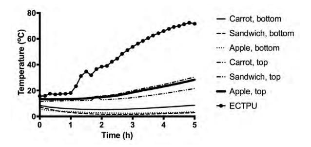
Figure 3. Exposure temperature for turkey sandwiches, sliced apples, and baby carrots packed in a cooler with a layer of ice on the bottom. Values represent the average temperature of three replications.
