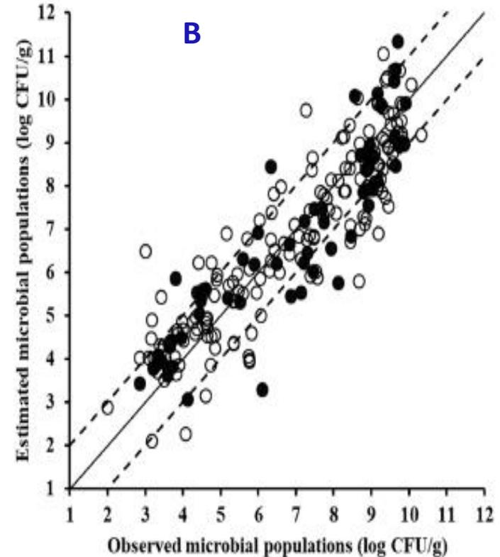
Training (solid symbols, 170 samples); validation (open symbols, 58 samples) datasets (solid line: the ideal  $y = x$  line; dashed lines: the  $\pm 1$  log; The root mean squared error (RMSE, log CFU/g) for the prediction of the test (external validation) dataset for the FTIR and VIS models was 0.915 and 1.034, respectively, while the corresponding values of the coefficient of determination ( $R^2$ ) were 0.834 and 0.788. 26
