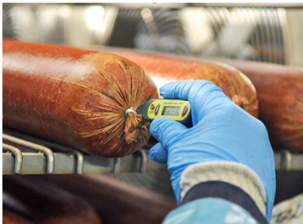
Figure 1. The monitoring procedures developed must take into consideration the nature of the product, type of processing equipment used and the device/tool used for monitoring the critical limit.
