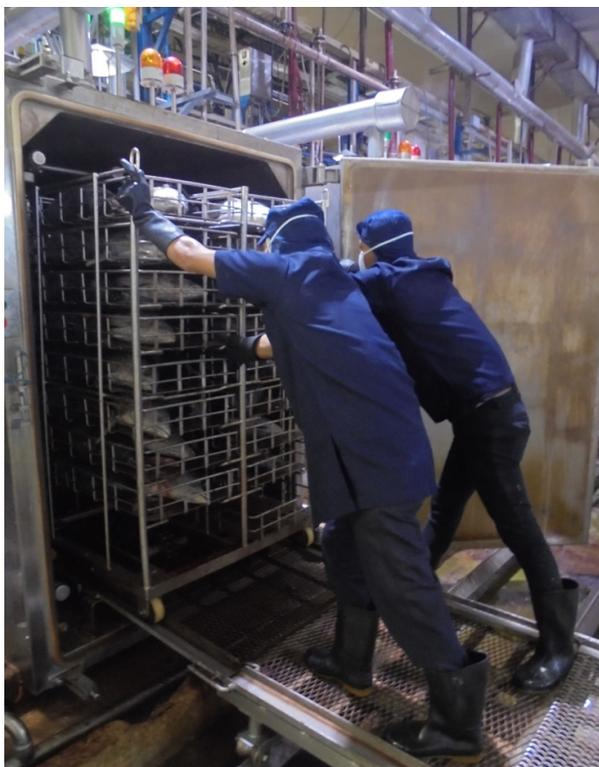
*Figure 1. A conventional atmospheric precooker*
