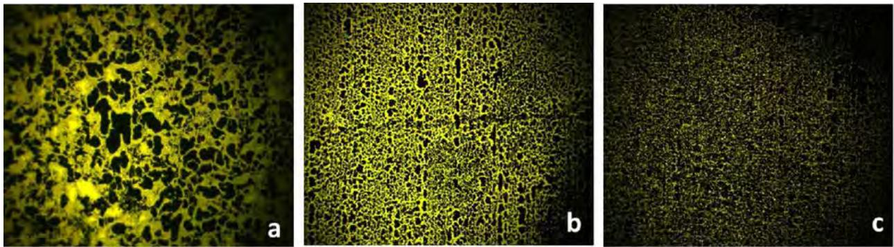
FIGURE 2. Microscopic fluorescent images, at 100× magnification, of stainless-steel coupons contaminated with biofilm, subjected to species/treatment conditions, and subsequently dyed using erythrosin B. (a) *Pseudomonas putida*/NT; (b) *Listeria innocua*/NT; (c) *Listeria innocua* /Enzyme.
