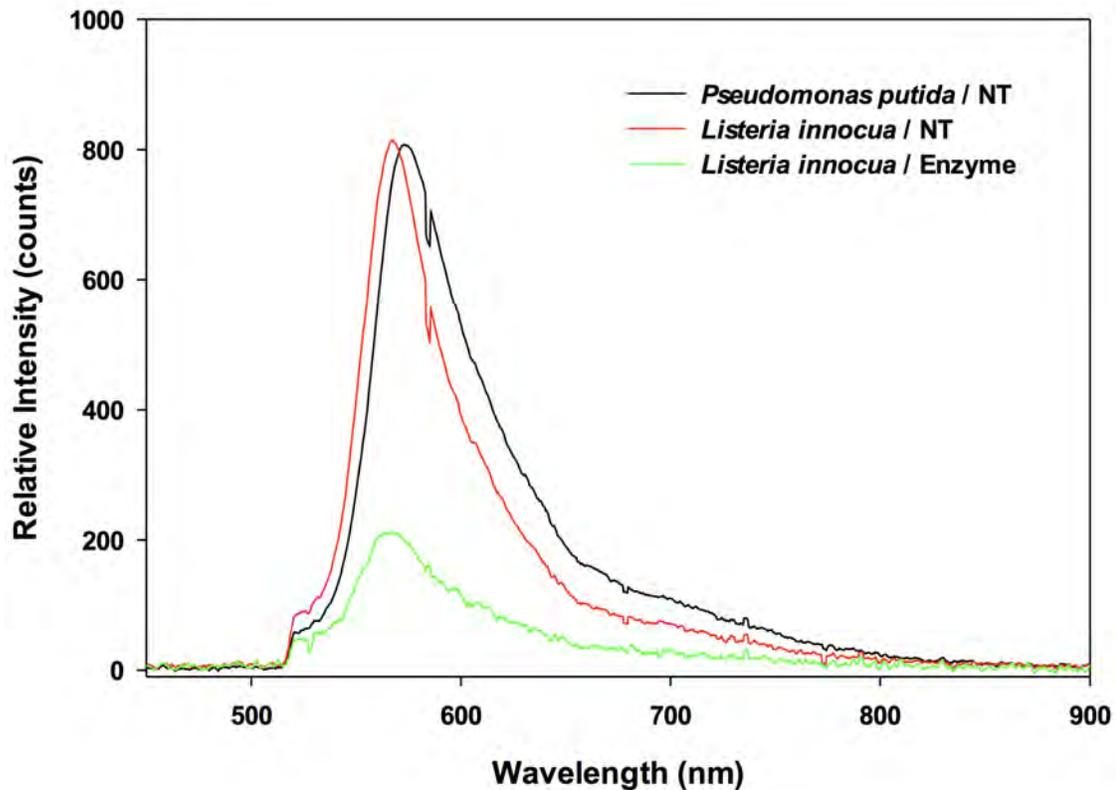
FIGURE 3. Fluorescence spectra of stainless-steel coupons contaminated with biofilm, subjected to species/treatment conditions, and subsequently dyed using erythrosin B.
