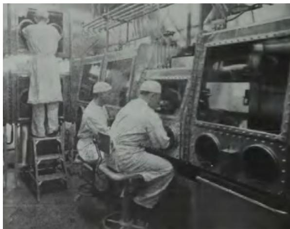
FIGURE 2. Research personnel working in a biosafety cabinet at Fort Detrick (p. 22, *Cutting Edge, A History of Fort Detrick 1943–1993*, N. M. Covert).
