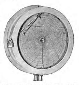
bottle switch on the outlet valve, or on both inlet and outlet valves where the milk is preheated, a time line is given on the chart which accurately checks with the temperature line.
