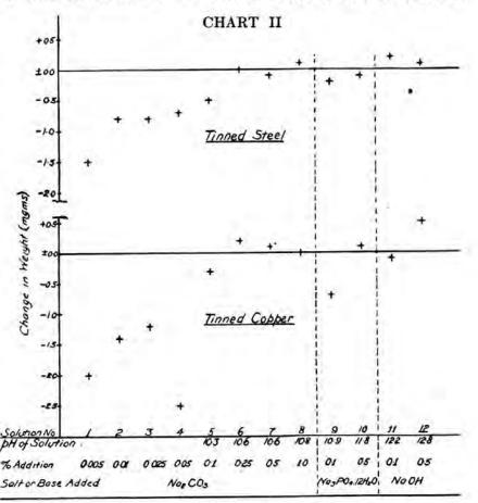
Changes in Weight of Tinned Metal Strips Half Immersed in Hypochlorite Solutions (100 hbm Available Chlorine) for 48 Hours at 30° C.
