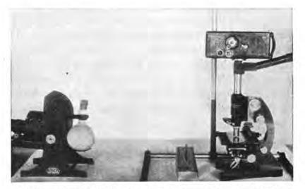
Equipment used to take photographs for photographic standard, using 35 mm. movie film.
