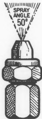
Wide Angle Cone Nozzle - Used for spot treatment on walls, ceilings and vegetation.
