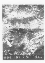
Figure 21. 2B finish glass beaded using 0.006 inch beads and 50 psi air
