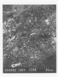
Figure 24. 2B finish glass beaded using 0.023 inch beads and 80 psi air
