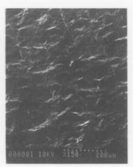
Figure 7. 60 grit finish stainless steel shat peened
