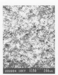
Figure 19. 2B finish glass beaded using 0.023 inch beads and 50 psi air
