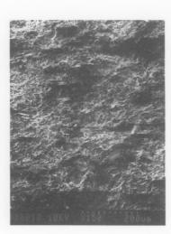
Figure 17. 2B finish glass beaded using 0.006 inch beads with 50 psi air
