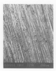
Figure 5. 2B finish stainless steel shot peened
