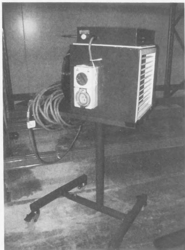
FIGURE 1. Hotbox-Axial HBA Fan Blower Heaters HB90415 – 415V 9.0kW used in heat holding chillers
